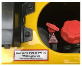
The **PURPOSE** of these identification items is to highlight to technicians that the engine oil should only be changed/topped up with the new specification of oil moving forward. The same applies to the driver/operator of the vehicle; only VDS-5 5W/30 engine oil should be used if topping up between scheduled service intervals.
