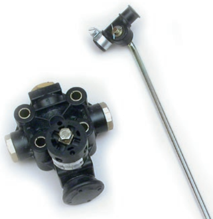
LEVELLING VALVE 4.0, PORTS: M12X1.5
